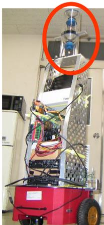
Omnidirectional camera on mobile robot
