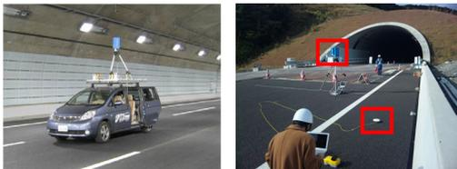
The 3D geometry inside the tunnel is scanned statically (stop-and-go) by every 20m. At the both ends, the scene including GPS antenna is scanned for several times.
