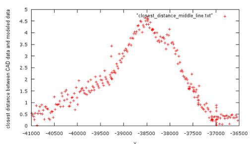
The closest distance between the tunnel midlines in 2D CAD data and our 3D data shows the largest difference exists around the central zone, which is no wonder since the error accumulation becomes maximum in the central. The amount is about 4.5 m, just 0.1% of the tunnel length in ratio. The second largest difference exist around  $x = -38000$  to  $-37700$ , which roughly correspond to the sharpest curve zone in a tunnel.
