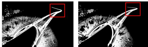
Multiple GPS data can fix absolute position and posture of the 3D models at the both ends. Simultaneous alignment is performed under this constraint kept, for global optimum.
