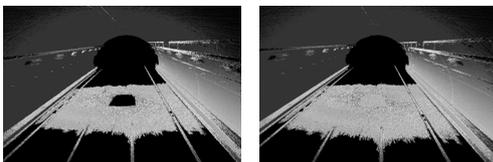
Deficient parts are filled by minimizing a cost function expressing that  $z$  values (point depth) become near to the scanned data when it exists, and are smoothly connected with surrounding data.
