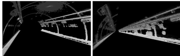
The partial 3D models acquired are locally stitched one-by-one using fast ICP calculation. For dealing with huge data more than 100GB, 3D edge features are extracted and used (reduced by 90%).
