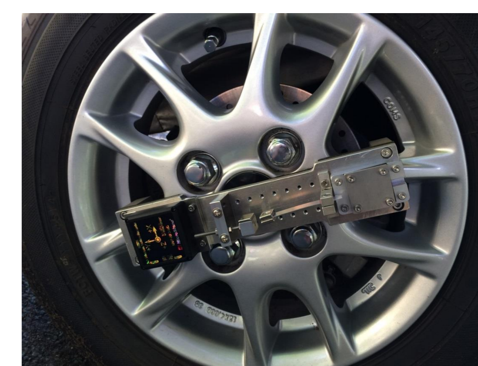
Energy harvester installed in the tire
