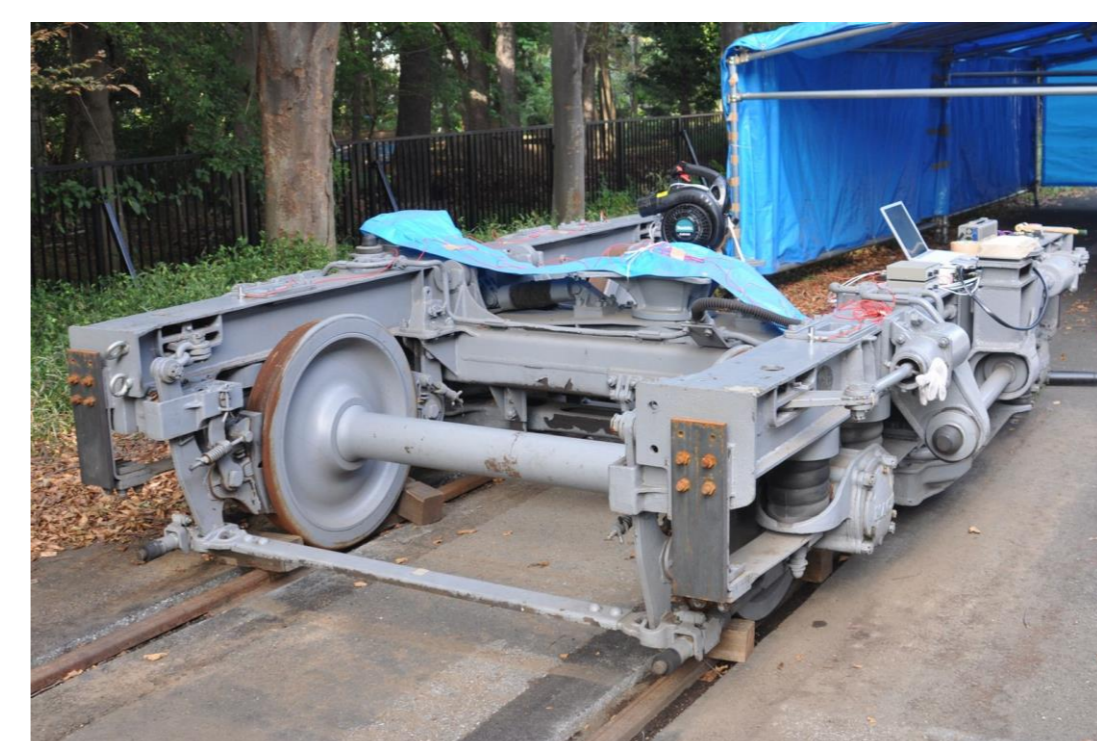
Vibration analysis on a railway bogie
