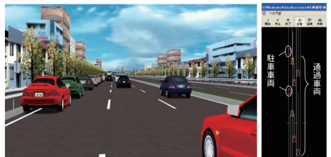
円滑性・安全性の観点に基づいた路上駐車による交通流への影響評価 Analyzing impacts of on-street parking on traffic flow in terms of efficiency & safety
