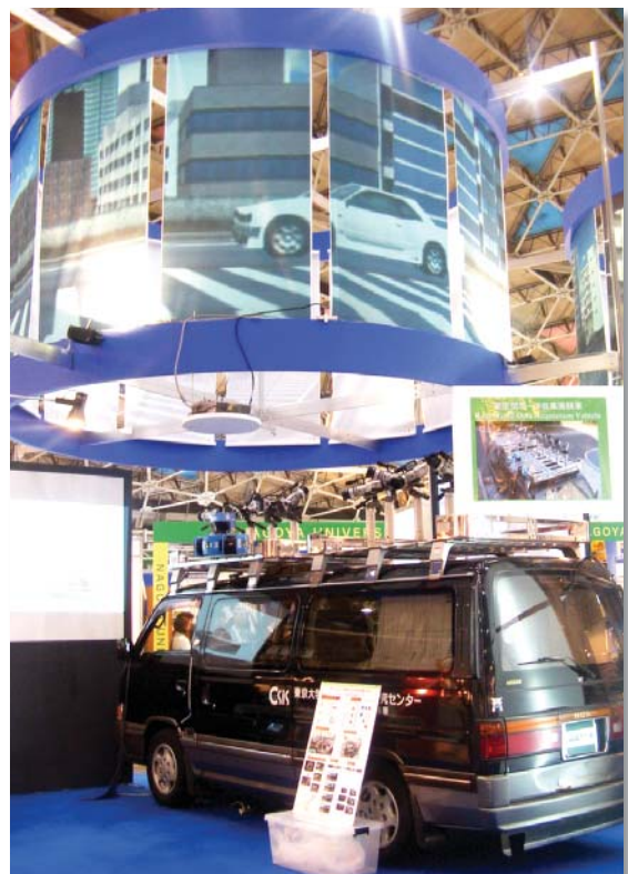
▲ Experimental "real space information collection vehicle" equipped with nine cameras.
