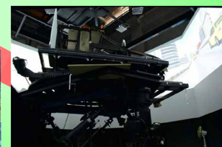
Driving Simulator with 6 d.o.f motion, Turntable & 360° Full Screen
